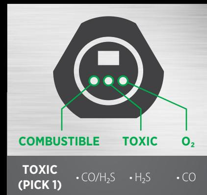
ALTAIR io360 Gas Detector use XCell<sup>®</sup> Combustible and Toxic sensors
